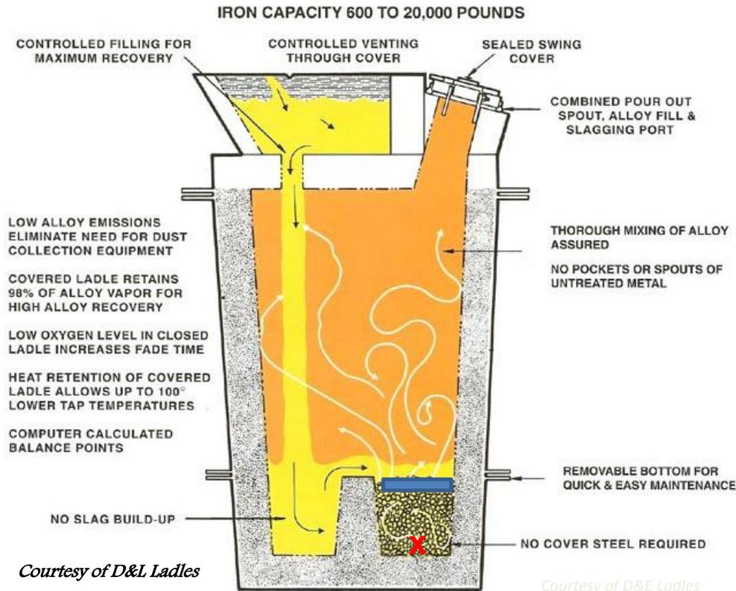
**X** denotes the location of Nodubloc in the bottom of pocket. The blue cover represents 1.2-1.5% Cover steel needed on top of pocket.
