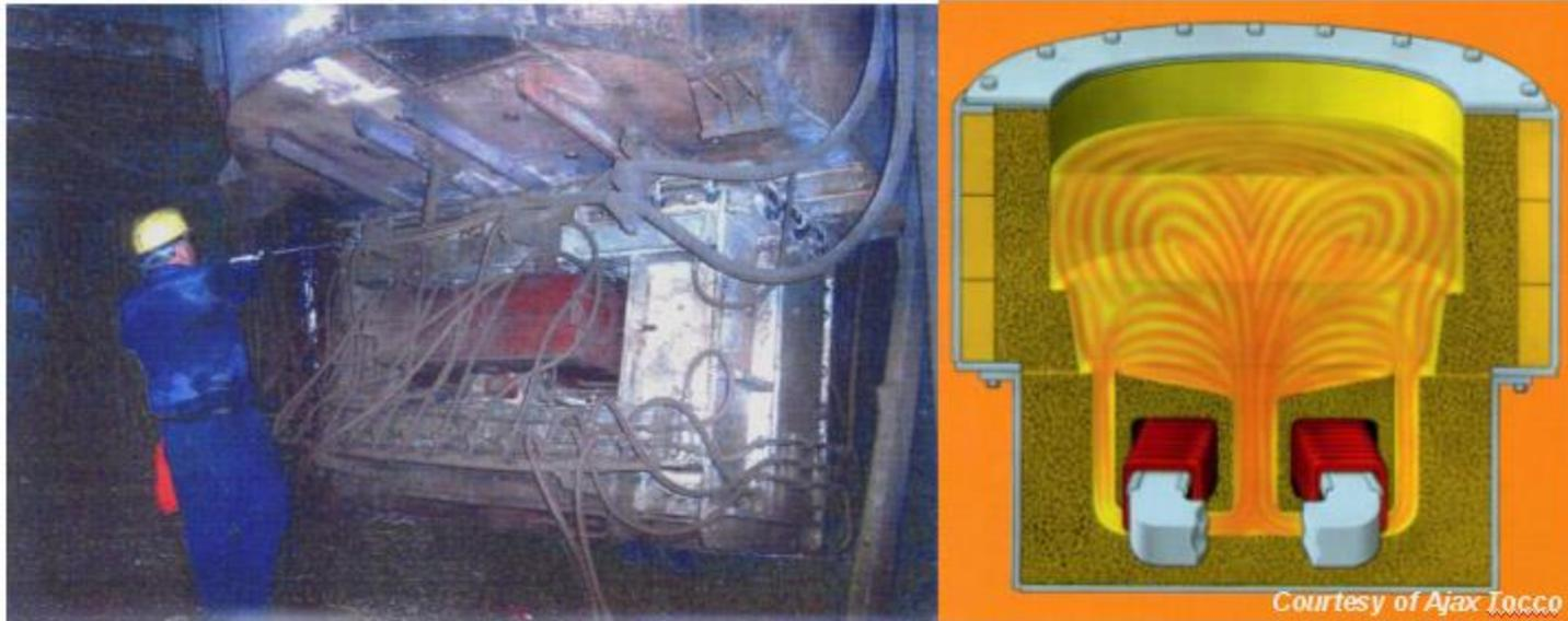
**Severe Restriction of Metal Flow in Throats or Inductor Channels can caused heavy saturation leading to refractory wear or metal leakage. Inability to superheat the molten iron.**
