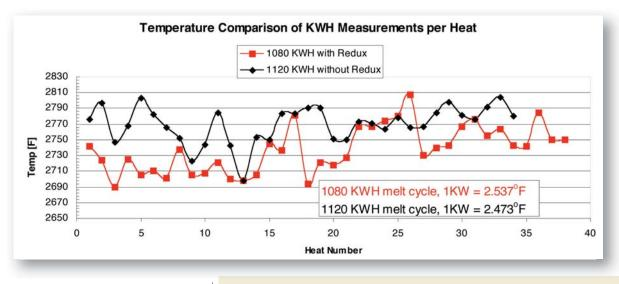
By incorporating two pounds of EF40L flux to each 4,650-pound charge, an immediate improvement in buildup reduction was observed. More importantly, it now requires only one kilowatt of power to increase temperature 2.537°F. Further, because slag buildup was so greatly minimized, Foundry T has reduced their kilowatthours per ton from an average of 1,120 KWH to 1,080 KWH, a reduction of almost 4.0% (see accompanying graph).
